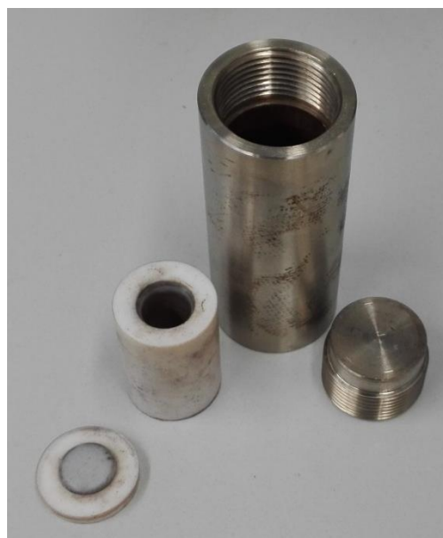
Figure C.01: Teflon®-autoclave (left) with lockable steel jacket (right)
