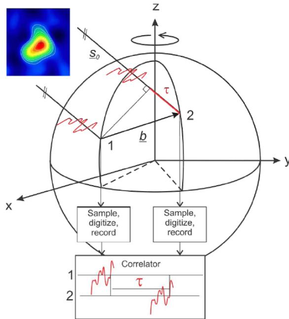
Figure 3.1: Geometric VLBI model.<sup>1</sup>
