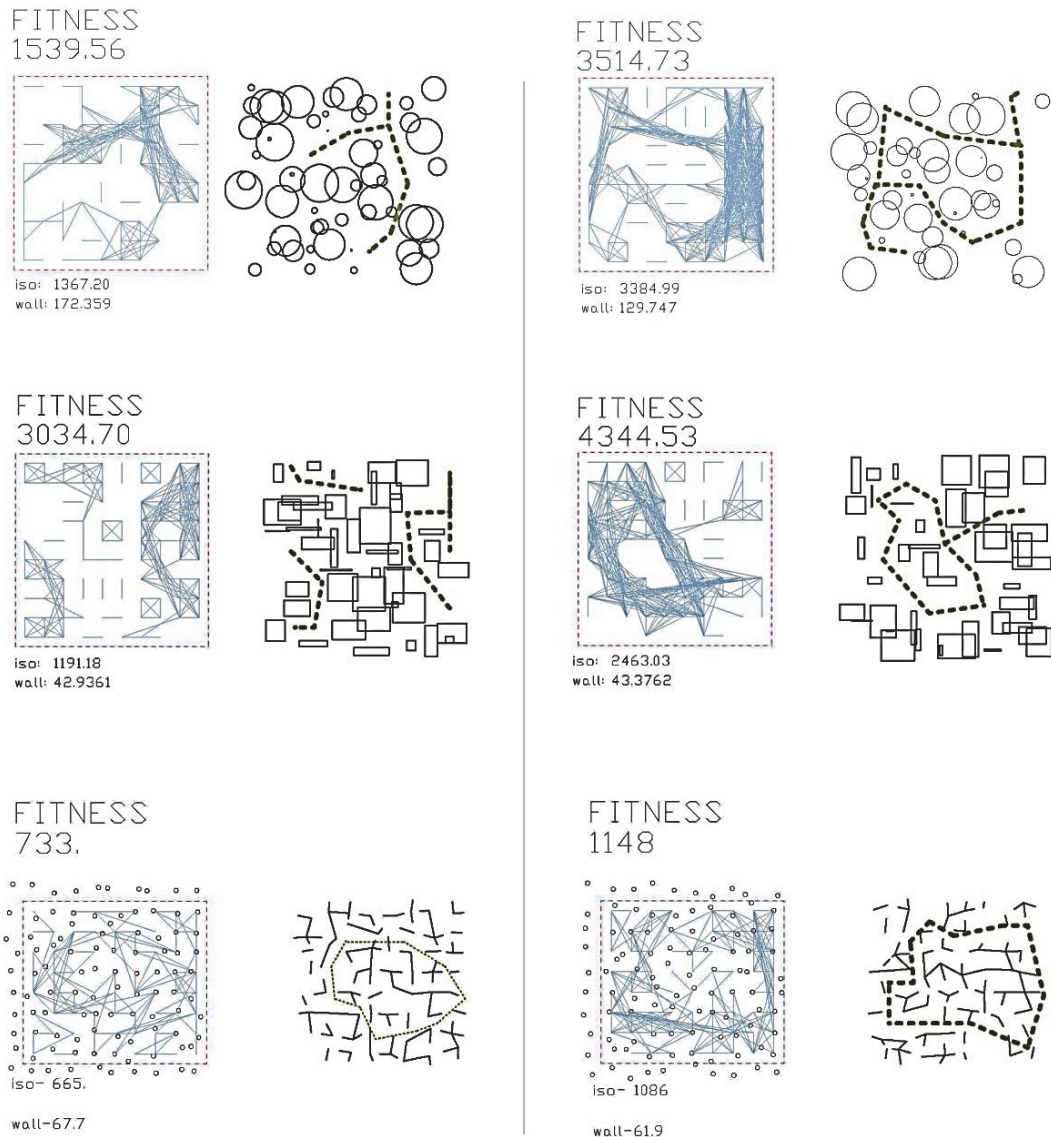
Fig232. Wall-2-Vision, Philip Langley (CECA), 2007: three randomized initial conditions (left) with varying geometric primitives evolve consistently ring-like circulation patterns with local clusters of spaces (right); the three experiments used slightly different fitness criteria, which shows in the top experiment creating larger mono-clusters
