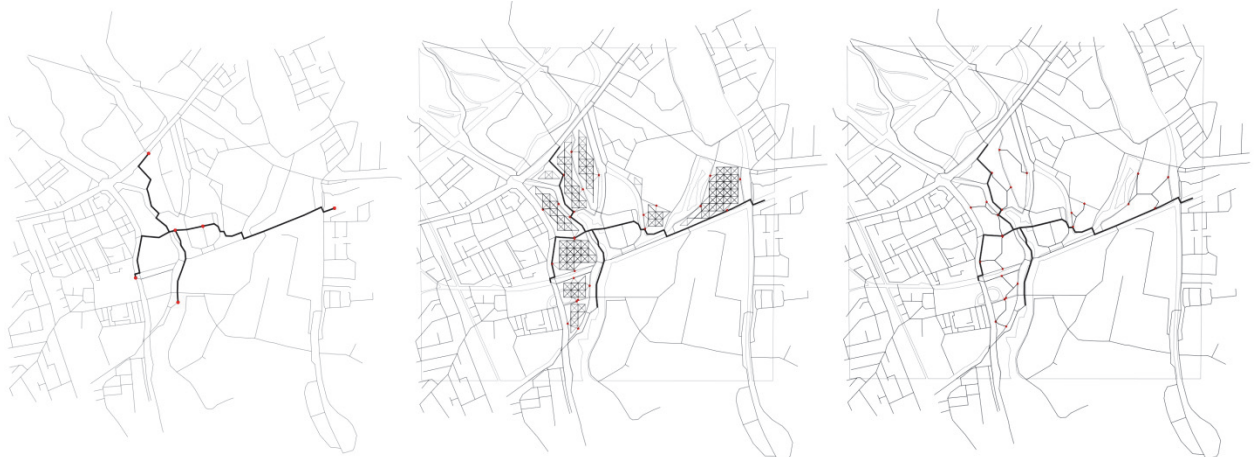
Fig175. Smart Solutions for Spatial Planning, 2008: (left) the primary street network tree graph generated from a k -MST; (middle) the primary network integrated into a generic grid of the total secondary network and (right) the resulting hybrid between primary and secondary networks
