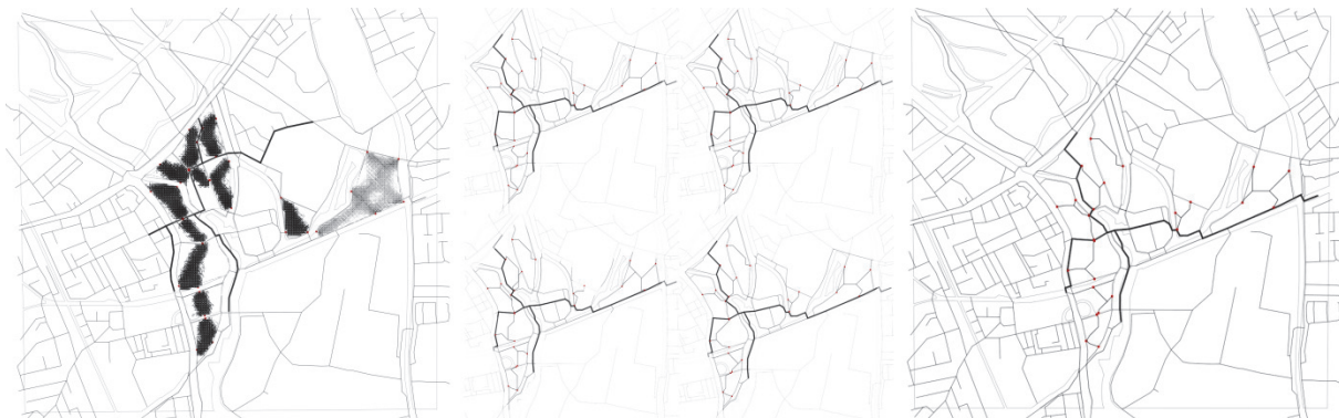
Fig176. Smart Solutions for Spatial Planning, 2008: (left) the ant-colony optimization algorithm (ACO) laying pheromone trails along the secondary network edges; (middle) four different states of the k-MST from ACO and (right) a final hybrid state of primary and secondary street network
