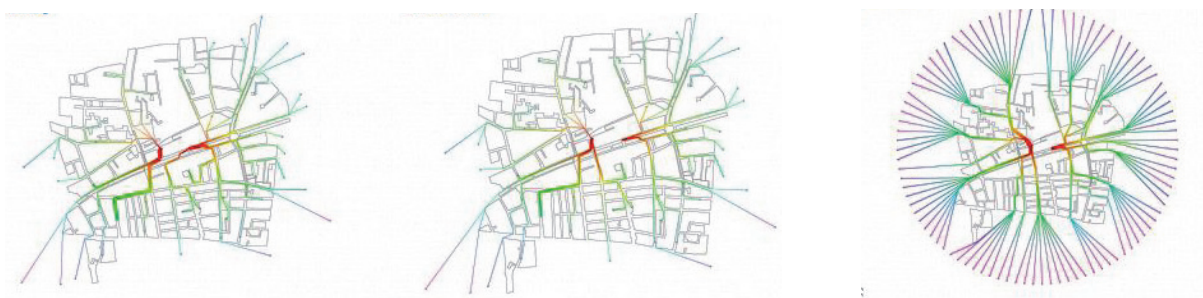
Fig169. Whitechapel CrossRail station crossing scenarios, 2009: (left) one extra and two extra crossings showing that one extra crossing does not enhance the walking times or add extra load to the eastern entrance; (right) same scenarios with extra noise added to flows via perimeter origin points
