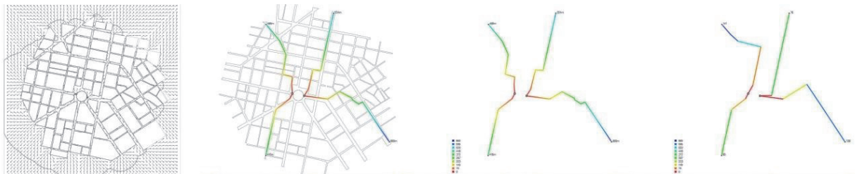
Fig167. Visibility Mesh to Graph: (left) flow field from the Field tool with four origin and two destination points; (middle left) metric shortest routes with same OD points; (middle right) the extracted graphs and (right) the two graphs weighted by least angular distance (which here are tree graphs)
