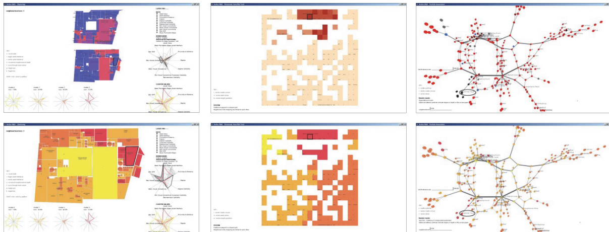
Fig223. IAA, RIBS, 2013: all analysis modes of a complex multi-floor layout such as here the Laenspar Banken, Falun. The left column shows the 1D SOM rendering the partitions (top) by asset values and (bottom) by all 10 spatial measures. The partition 'customer vault' is selected in the 'red' cluster, which contains 12.2% of all rooms, i.e. 12.2% of all partitions have a similar quality; the middle column shows the 2D Mnemonic SOM distribution of partitions with (top) the asset values rendered and (bottom) the cluster numbers rendered; the 'customer vault' partition is in the centre of the 'red cluster', showing that it does not interface with any other cluster partition; the right column shows the 3D permeability topology, clearly visualizing the circulation cycles and the outliers as according to Hillier's space types; also visible are the more 'risky' or high value assets are deeper and away from the main circulation cycles and the 'customer vault' partitions are set-off from the main circulation little accessible
