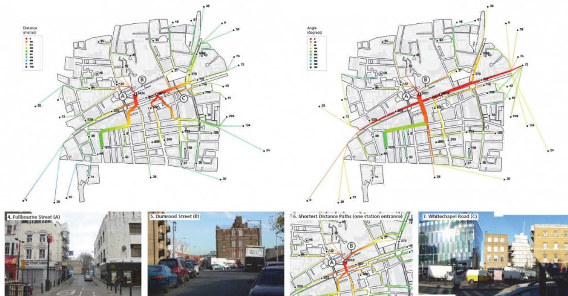
Fig168. Whitechapel CrossRail station entrance configuration analysis, 2009: (left top) two entrances catching approximately 50% of commuters and showing that envisaged small alley behind station site might not generate footfall (b); (top right) least angle analysis providing insights for flows from hospital for out-patients and potential new crossing
