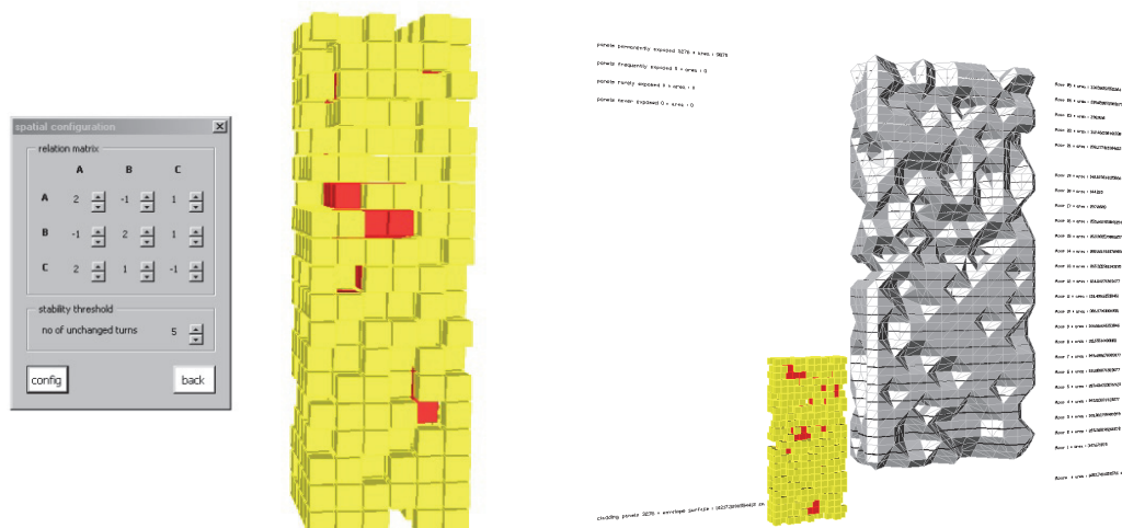
Fig85. Faulty Towers Stage A Cellular Automaton allocating programme across the topologically partitioned volume (left) and its stage B geometric translation (right)
