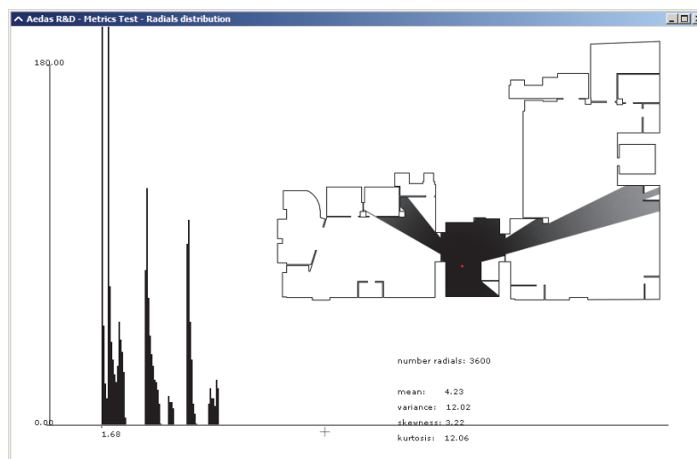
Fig65. Single isovist from the red node, showing four of Benedikt's measures and a distribution histogram at the bottom of radial lengths; developed by Aedas CDR for the RIBS projects, 2010 (6.1)
