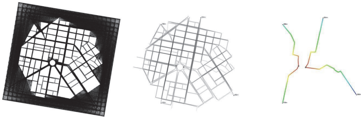
Fig166. Visibility Mesh to Graph: (left) visibility graph as produced by VGA on a site in Athens (with students of IE University, 2013); (middle) visibility graph generated from geometry vertices only and (right) shortest routes graphs from same OD points shown in the middle visibility graph
