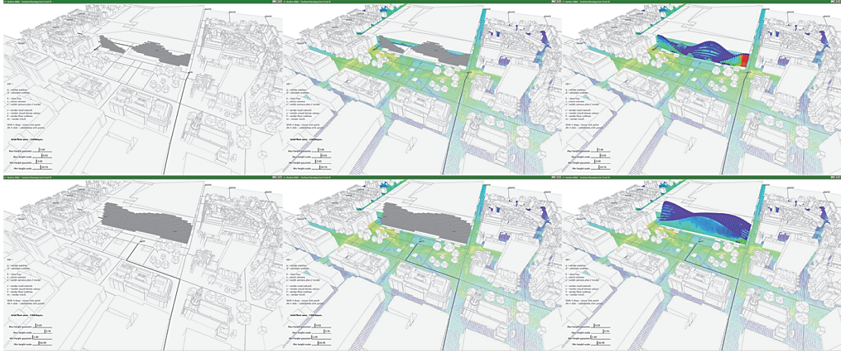
Fig250. Euston Pilot, 2013: two massing states by changed access points and Gaussian distribution weighting producing very different building mass performances
