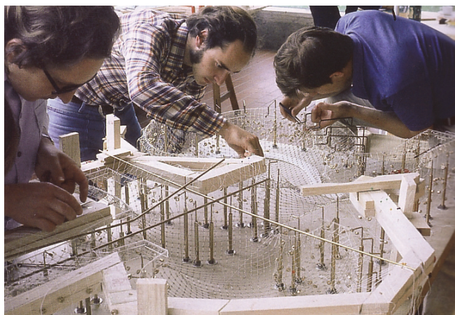
Fig323. Frei Otto, 1960s: catenary and tensile models represent 'live' material computation whose behaviors are autonomous from the user who has to interact to learn their dynamics (Otto and Rasch 1995)
