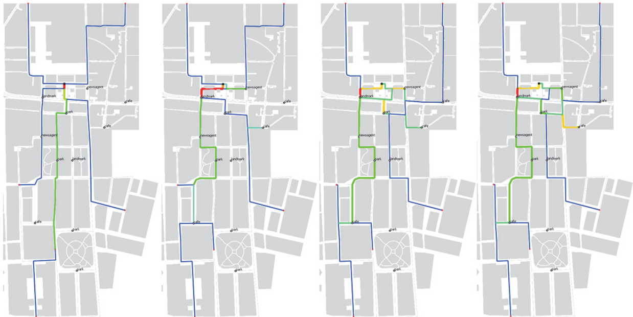
Fig229. Four instances of an access network for the Euston Crossing project (7.2.2): the network is weighted from 0% (left) to 100% (right) to approximate individualistic behaviours by routing origin points to a destination point through preferred locations such as cafes, newsagents and others; the standard 0% deviation graph represents shortest routes and the colours indicate the flow load along graph edges when preferences change
