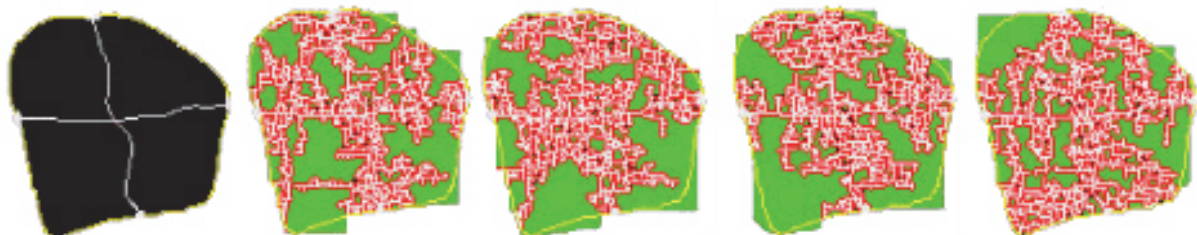
Fig275. Paul Coates, 1999: the Sanaa model implementing the 'alpha syntax' for a CECA student; (right) seeded north-south and east-west axes and a series showing growth stages with white cells as street, red as solid and green as gardens (Coates and Derix 2007)
