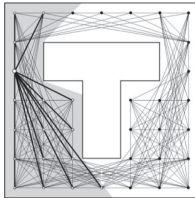
Fig62. The visibility graph constructed from a discretized area grid by Alasdair Turner (Turner et al. 2001)
