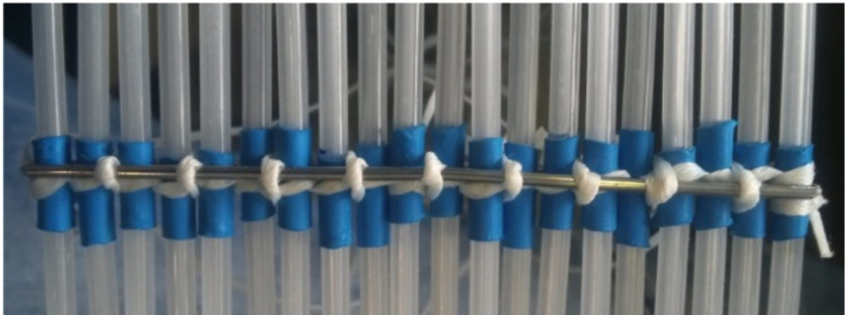
Figure 2.6: Connection of a flat cable layer by lacing cord, reinforced by metal pins 35
