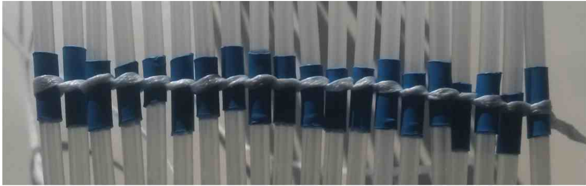
Figure 2.5: Connection of a flat cable layer by lacing cord 34
