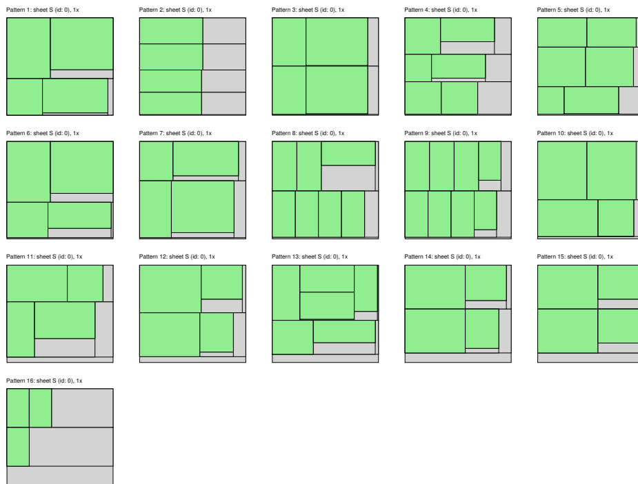
(a) Solution to instance CU9 using DP-Generator, with symmetry = 1.
