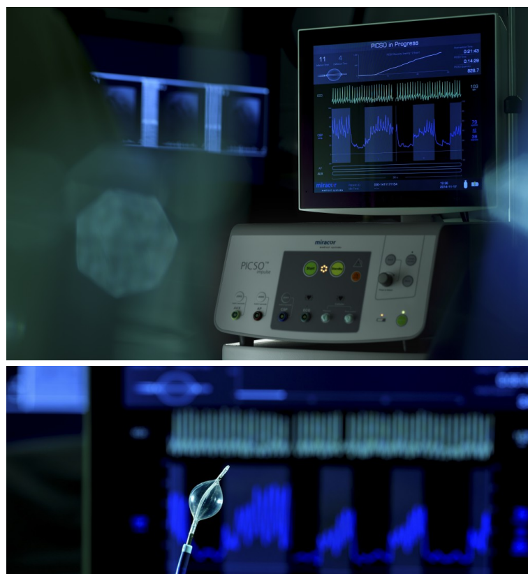
Figure 5.5: PiCSO AMI Impulse Console (above): The monitor displays the inflation / deflation state of the balloon, as well as trend graphs and time counters; Live graphs display curves and numeric values of ECG, CSP, AP and auxiliary input. PiCSO Impulse Catheter (below): 8 French triple-lumen catheter with a low profile, semi-compliant balloon and an atraumatic distal tip. It is inserted in a standard over-the-wire technique via the femoral vein and placed in the coronary sinus using a steerable guide sheath. Two marker bands show the extension of the balloon in the coronary sinus [Miracor Medical SA (2018)].
