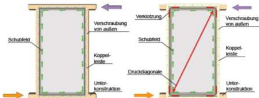
Abb. 2.17 (li.): System HFA – Schubfeld [31]
