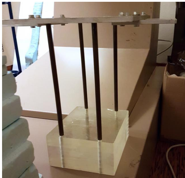
Fig. 3.4: PMMA block for irradiation of farmer chamber and TLDs. The block was mounted at 30 cm distance from the ^{60}\text{Co} source.
