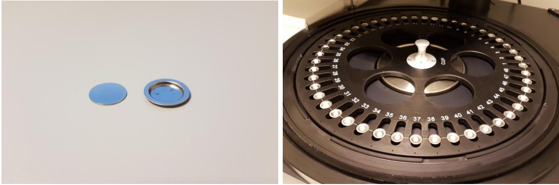
Fig. 2.5: Sample holder in form of disk and cup (left) and sample wheel for cups (right)
