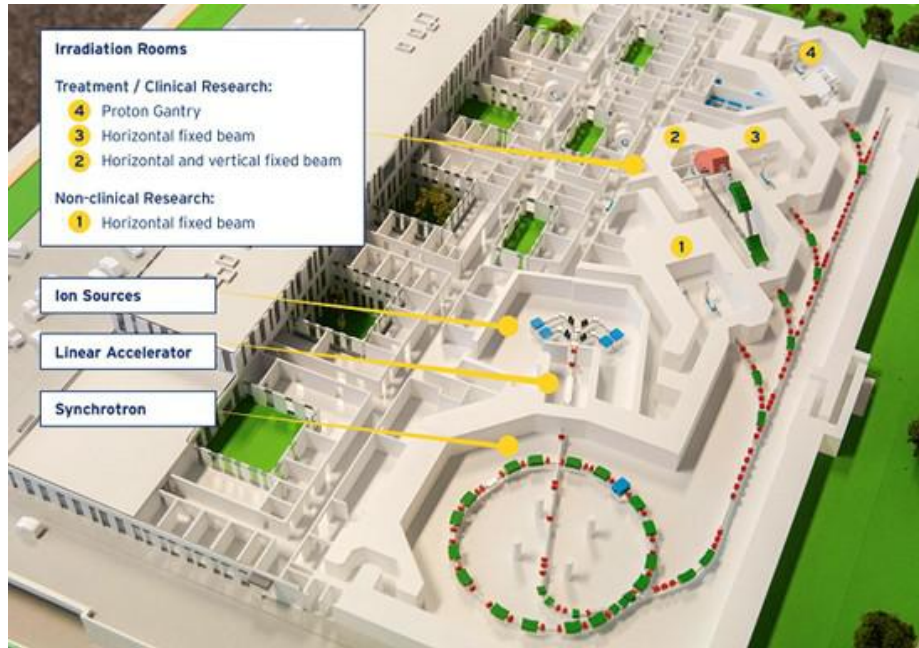
Fig. 1.8: 3D model of MedAustron with accelerator and irradiation rooms (source: [24])
