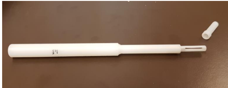
Fig. 3.3: TLD holder in shape of the farmer chamber. At the tip of the holder three TLDs can be placed next to each other in the small slit
