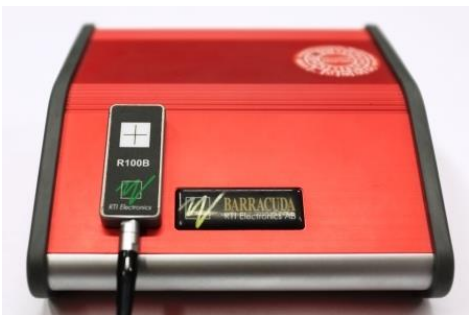
Figure A.3: Barracuda with dose probe R100B
