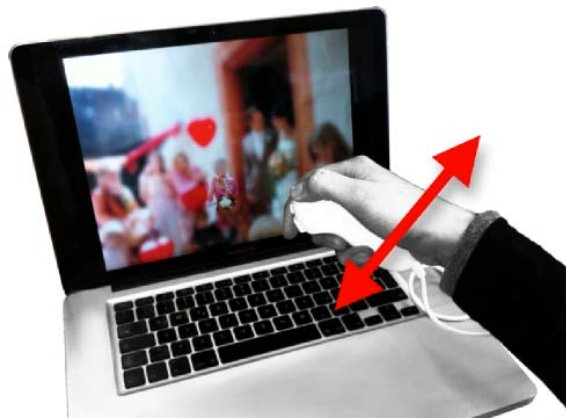
Figure 5.4. Navigating the clear spot of EyeOfDetail by moving an accelerometer input device.
