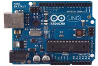
Figure 3.1. Arduino microcontroller board for fast prototyping of physical computing devices. (Stoneburner, 2010).
