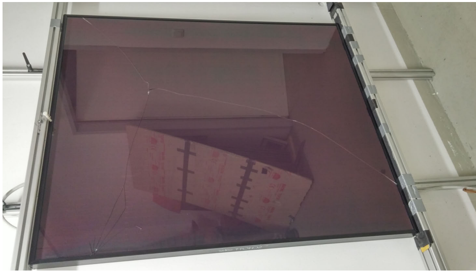
Fig. 3.47: The a-Si module is shown from the front side and therefore mirrored vertically to match the back side measurements. Each cell has a width of 19 mm.
