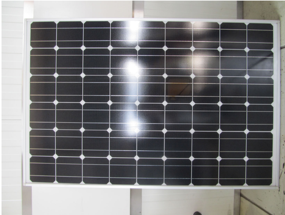
Fig. 3.53: The mono c-Si module is shown from the front side and therefore mirrored vertically to match the back side measurements. There is visible browning of a central cell.
