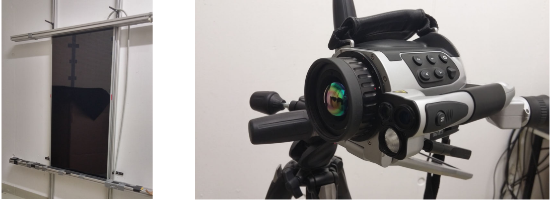
Fig. 3.2: PV modules are mounted to the wall by using aluminium profiles. The reflexion on the module shows the reflexion shield. The thermocamera is shown on the right (see text).
