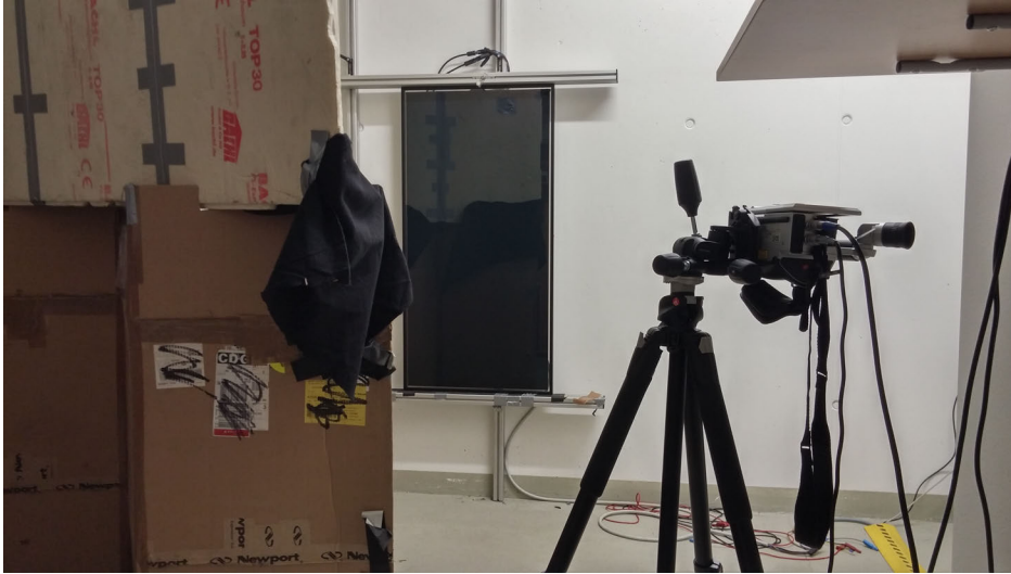
Fig. 3.6: The thermocamera is elevated by a stand on the right side. On the left is the reflexion shield made of cardboard and styrofoam, stucked together with some type. Black felt cloths are put upon leaks in the shield.
