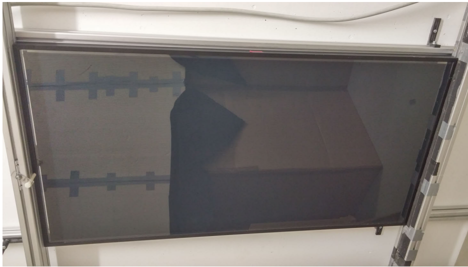
Fig. 3.42: The CIS module is shown from the front side. Each cell has a width of about 4 mm.
