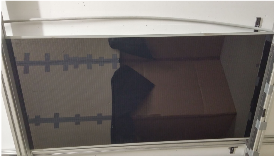
Fig. 3.35: The CdTe module is shown from the front side. Each cell has a width of about 1 cm.
