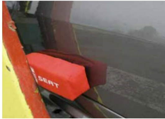
Abbildung 24: Magnetischer Türschutz (aus Finished Vehicle Logistics Magazine 2/2012, S.58)
