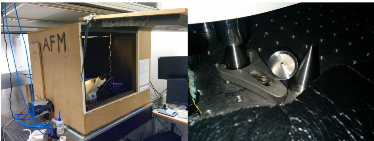
FIGURE 4: A WOODEN BOX (LEFT) DAMPS VIBRATIONS TRANSMITTED VIA AIR. STEEL CONES (RIGHT) MOUNTED UNDER THE MICROSCOPE DECOUPLE IT FROM VIBRATIONS TRANSMITTED VIA THE TABLE.
