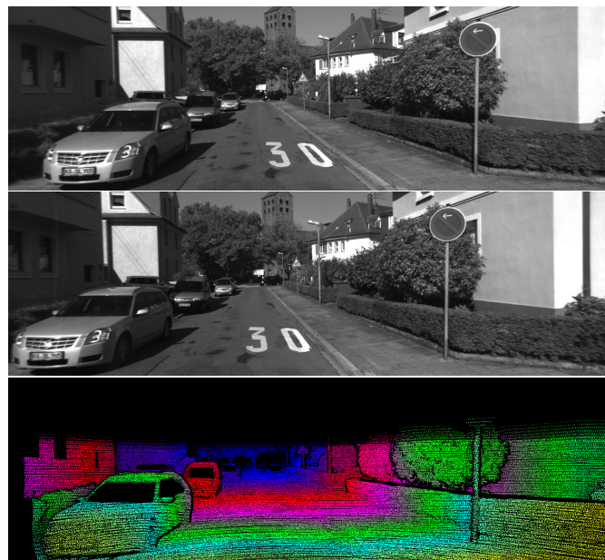
Figure 5.1: Left and right stereo image pair 110 of the Kitti Vision Benchmark dataset [17], together with the color-coded ground truth disparity map for the left image (yellow: close, blue: far away, black: no ground truth data available).
