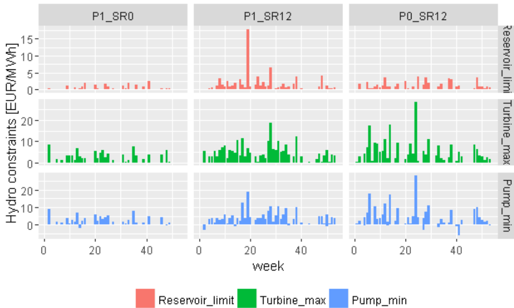
Figure 3.30.: Maximum prices of hydrological constraints as a result of the capacity reservation for positive balancing power.
