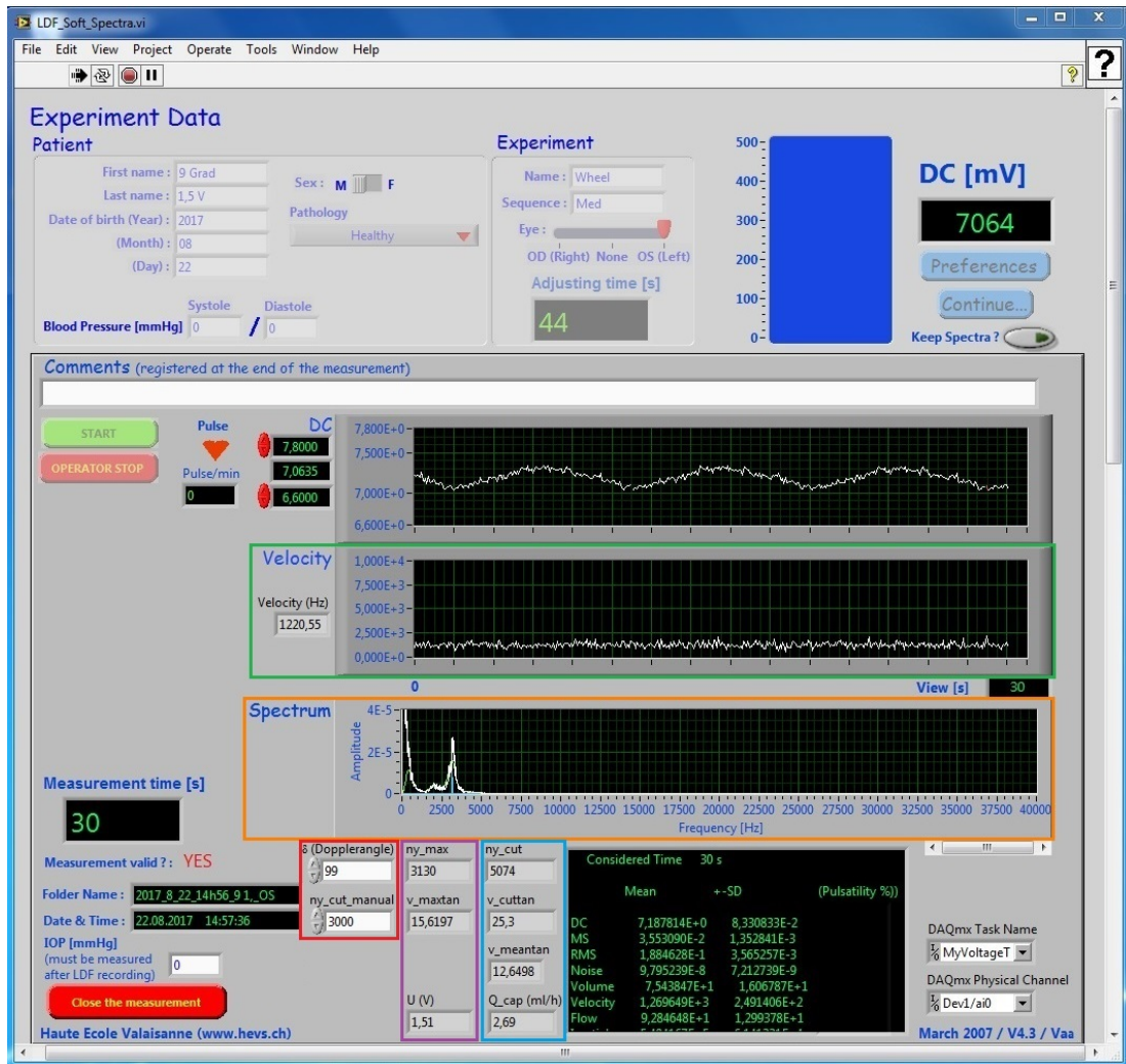
Figure 4.8: Changed measurement screen of the LabVIEW program. The second display shows the development of the average velocity (green rectangle) and the third display shows the averaged spectrum during a measurement (orange rectangle). Also included in the third display are several graphs for results derived from the averaged spectrum. The two controls are needed as additional input during measurements (red rectangle). The two columns of three and four indicators are for results of the different experimental setups (violet and blue rectangle). They are further described in Chap. 6.
