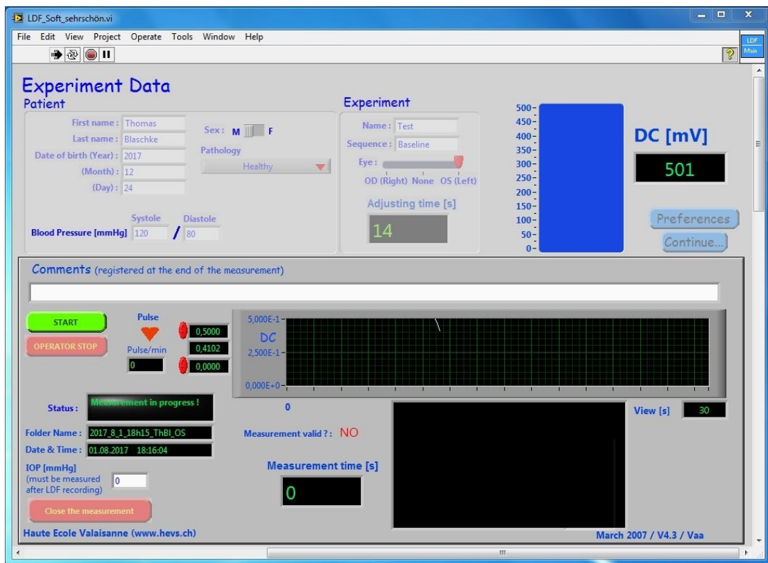
Figure 4.5: Measurement screen of the program with the visible program elements used for a measurement after clicking the "Continue..."-button on the input screen.
