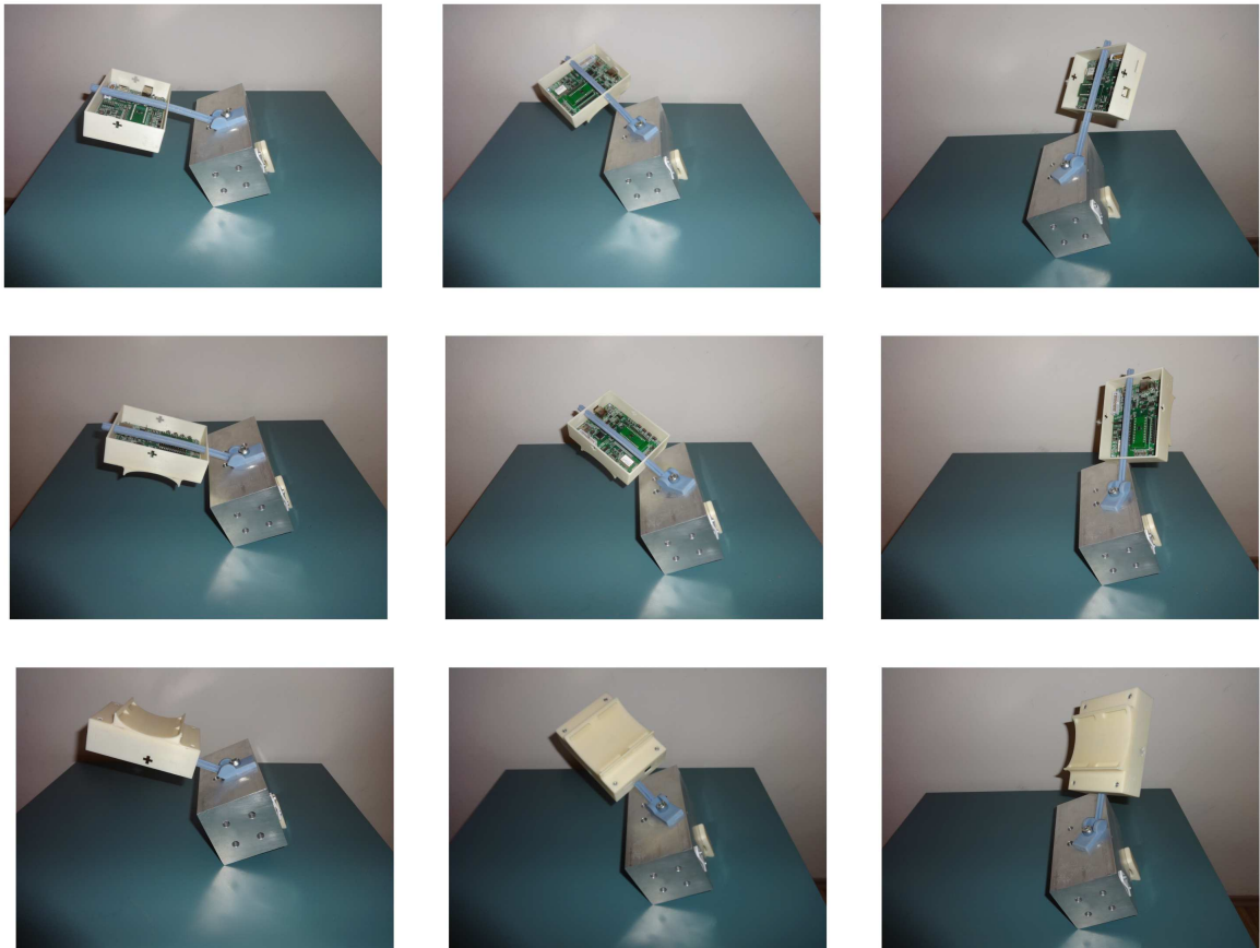
Figure 5.2: Example measurements of the gravity reference vector in different orientations in static state using the calibration equipment.
