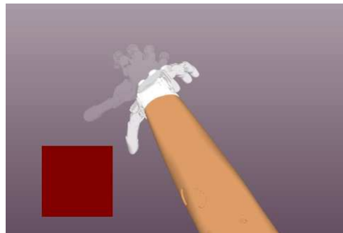
Figure 5.11: During this test, the virtual prosthesis has to be moved into the target configuration illustrated by the semi-transparent hand.
