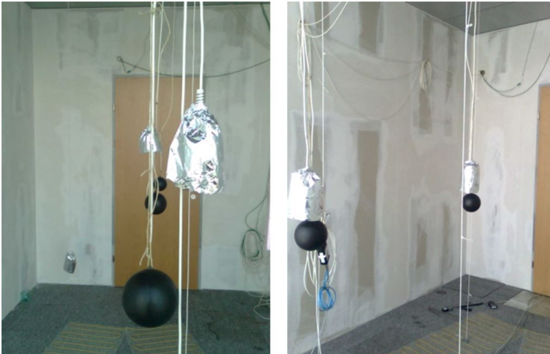
Figure 2.14: Photo of the measurement of the air temperature and the humidity; LinPicco; no direct radiation on the sensor
