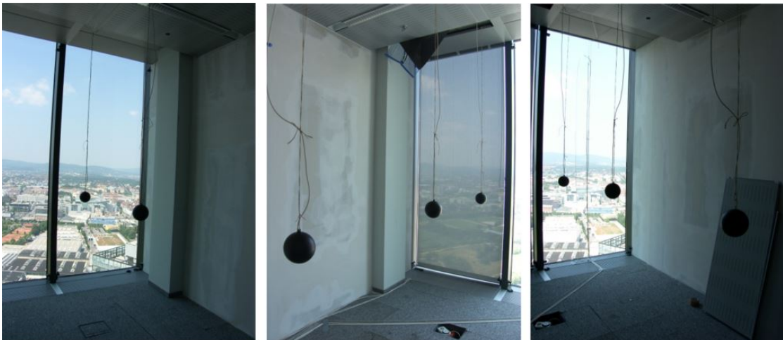
Figure 2.19: Pictures of the measurement of operative temperature; in the picture it is seen that the measurement was done with black balls (PT1000 sensors inside; diameter of 100\text{ mm} ) in 3 depths of the room
