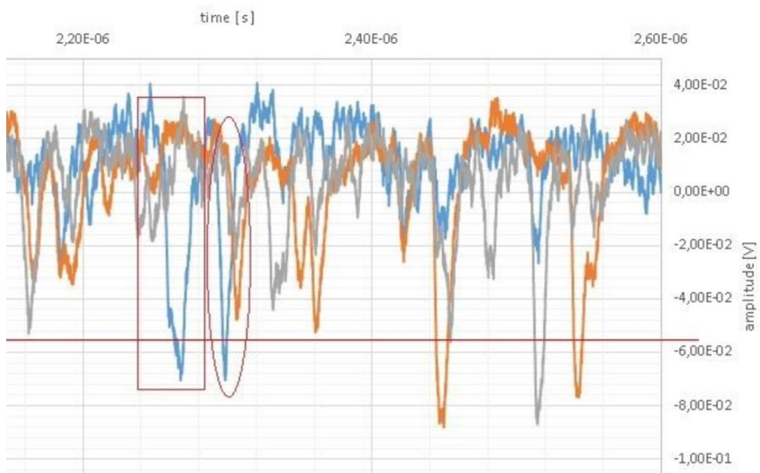
Figure 8: The pulse-height spectra plotted for slow antiprotons, which arrived in a time window between 2.0-2.6 \mu\text{s} . The three lines (blue, orange, gray) correspond to the three different SiPMs, respectively.
