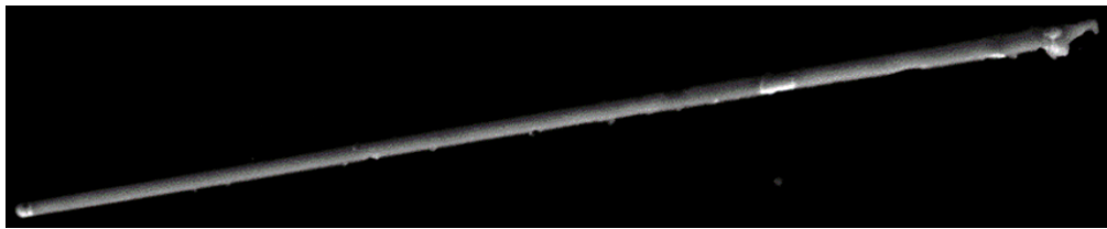
(c) Si-Au NW heterostructure after the third FLA process
