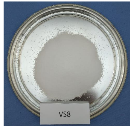
VS8: fine, 95 mg/kg Sodium ferrocyanide
