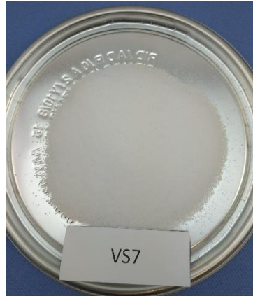
VS7: fine, 22 mg/kg Sodium ferrocyanide
