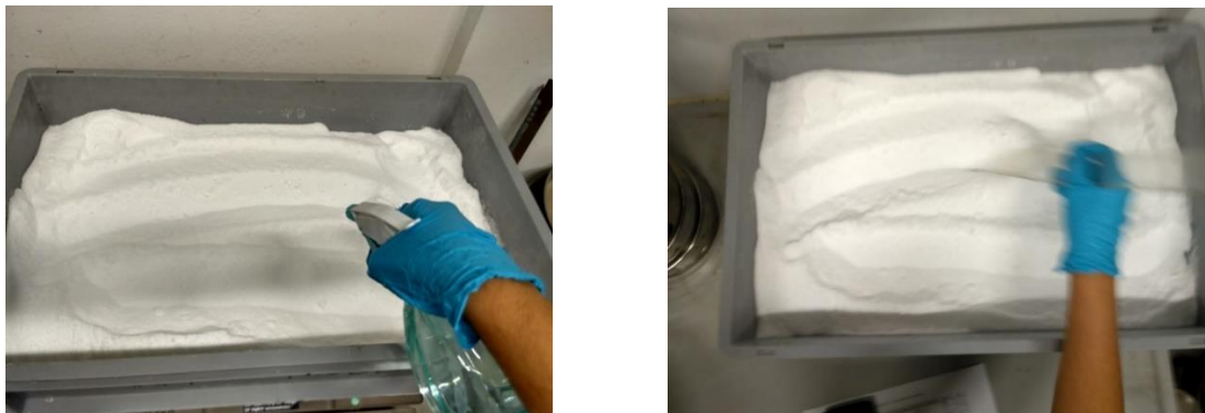
Figure 10: Sample preparation - water spraying
