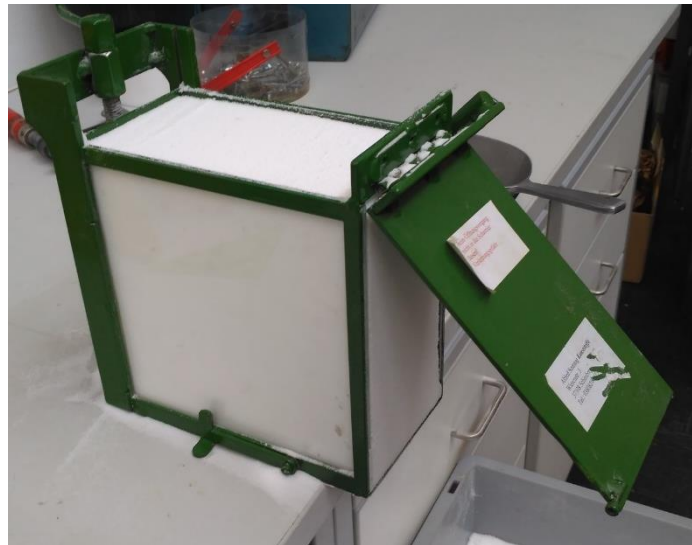
Figure 28. Auslaufbox with 0% outflow
