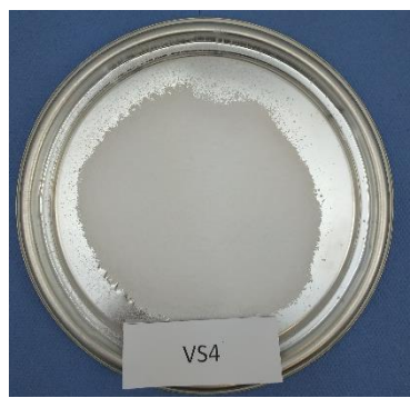
VS4: fine, 8 mg/kg Sodium ferrocyanide
