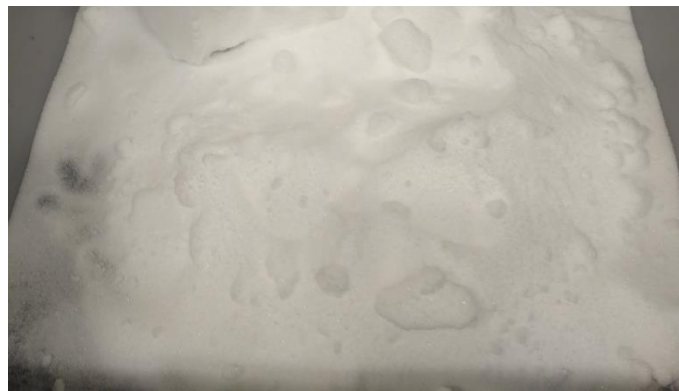
Figure 29. Sample VS3 with lumps from caking
