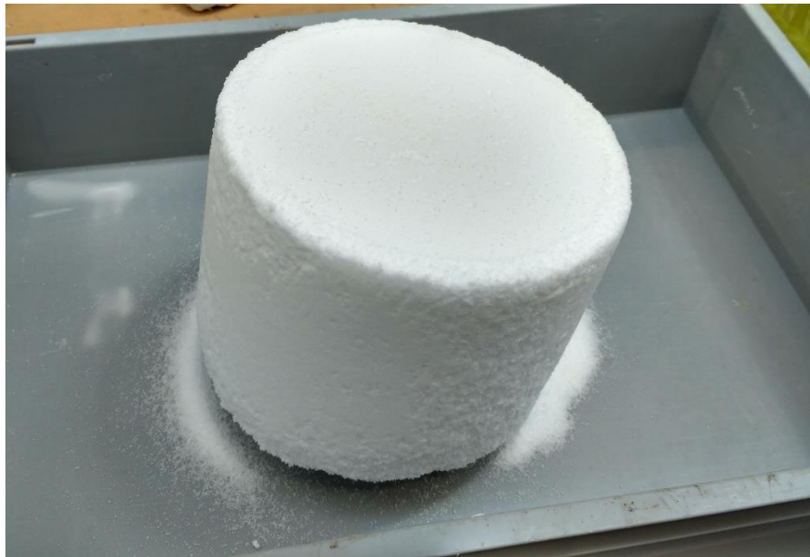
Figure 23. Sample VS2 after being dried in the oven, forming one big lump
