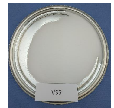
VS5: fine, 8 mg/kg Sodium ferrocyanide
