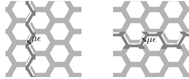
Figure 2: Two types of lineic defect: the zigzag and the armchair cases
