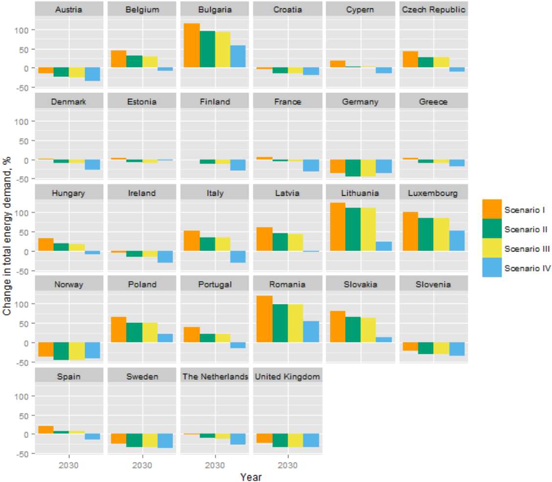
Fig. 64 Change in total energy demand for space heating, cooling, appliances, ventilation, refrigeration and lighting in Shopping Centres from 2012 to 2030 in the European countries in different scenarios
