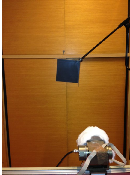
Fig 111: Acoustic retro-reflector built from three sound-hard planes. The acoustic-retro reflector was located from multiple positions on the belt. The calculated reflection points are all very close to each other with a total point-spread of approx. 9 mm.
