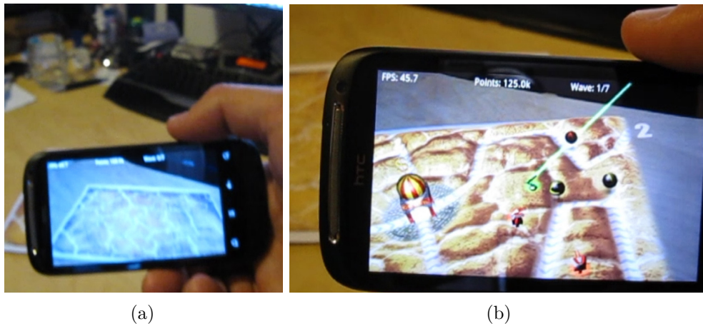
Figure 2.24: An AR tower defense game created by Michael Probst and Johannes Unterguggenberger for the course Augmented Reality on Mobile Devices on Vienna University of Technology in 2011. It uses Vuforia tracking SDK to find the image target, shown in (a). The image target looks like a dry cracked desert ground and has many image features like sharp corners and high local contrast which Vuforia is able to track well. Once Vuforia has recognized the target, it provides a pose matrix. The game uses it to render the battlefield atop the image target like shown in (b).
