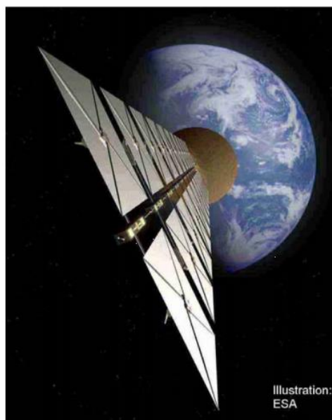
Figure 6: SPS concept in GEO - European Sail Tower (Seboldt, 2004)
