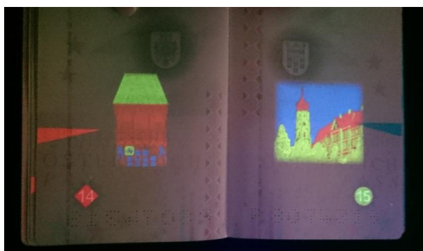
Figure I.B.4: Austrian Passport under UV-light, secured by the luminescence of various Ln-compounds
