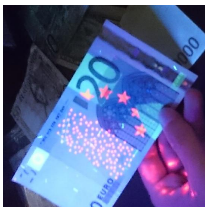
Figure I.B.4 A 20 Euro note under UV-light, secured by luminescence of Eu-oxides
