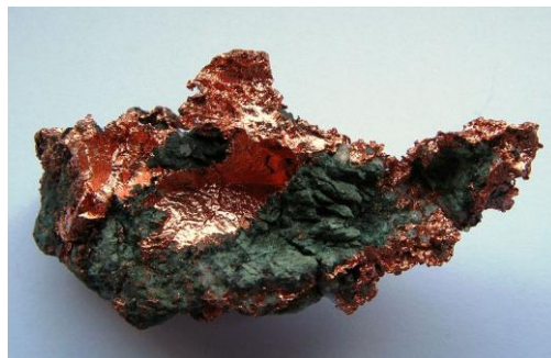
Figure II.A.8: Native copper mineral with impurities from other elements and oxidation processes [40]
