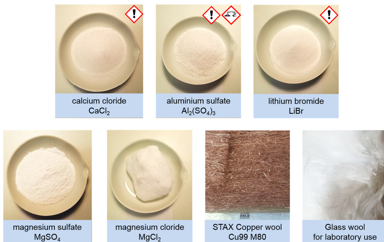
Figure 28: materials in use to create TCHS composites [10]
