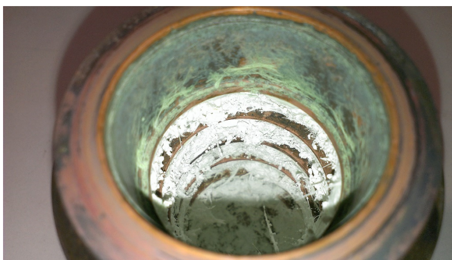
Figure 37: view inside the reactor after 14 use cycles (sorption/desorption)
