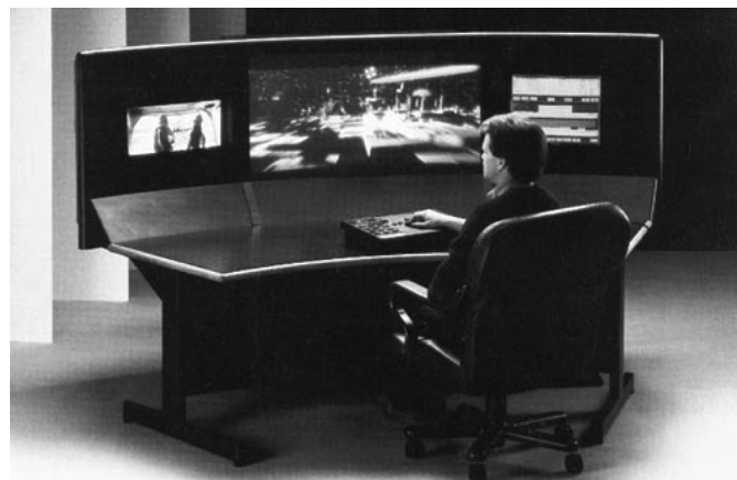
Figure 3.11: EditDroid was developed by LucasFilm and used Laserdiscs to allow fast random access to any frame in a video sequence.
