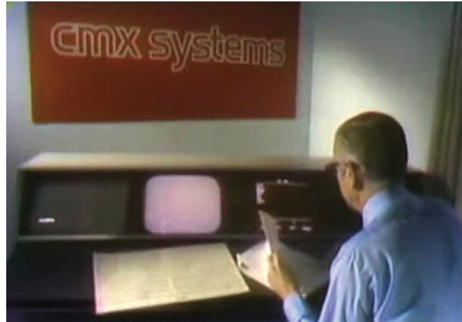
Figure 3.10: The CMX 600 was the first non-linear video editing system allowing the operator to access any frame in a 30 minute video sequence within 1 second.
