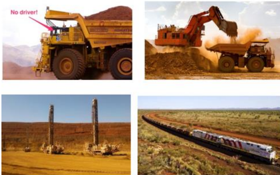
Figure 24. Autonomous dump truck; Autonomous excavator; Autonomous drills; Autonomous train (from left to right). (Burke, 2016)
