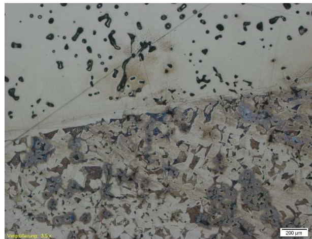
Figure 118 Interface between MA and substrate. H45_E13
