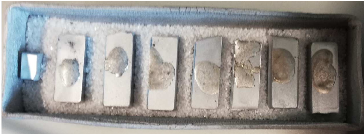
Figure 14 Wetting samples after the furnace run
