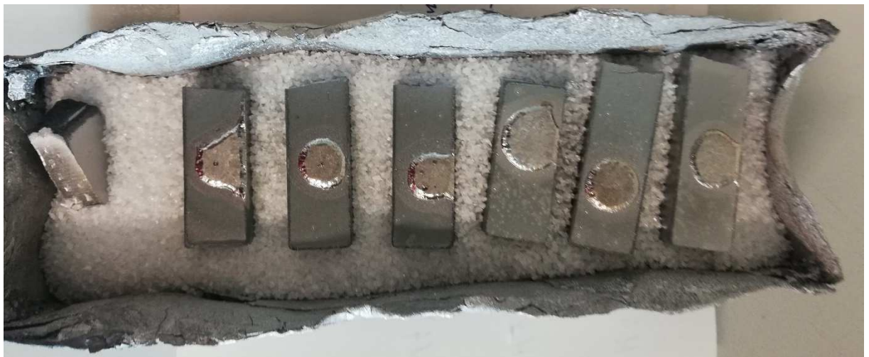
Figure 16 Infiltration samples after the furnace run
