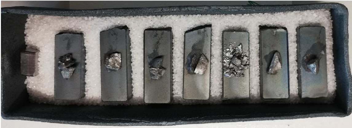
Figure 13 Wetting samples before the furnace run
