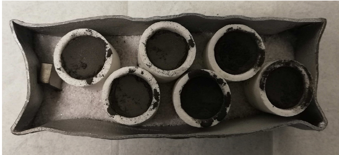
Figure 6 LECO crucibles filled with powder mixes
