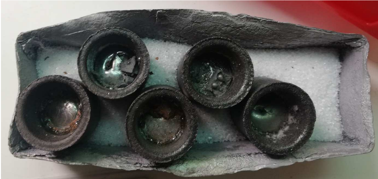
Figure 7 Powder mixes molten to ingots after furnace run
