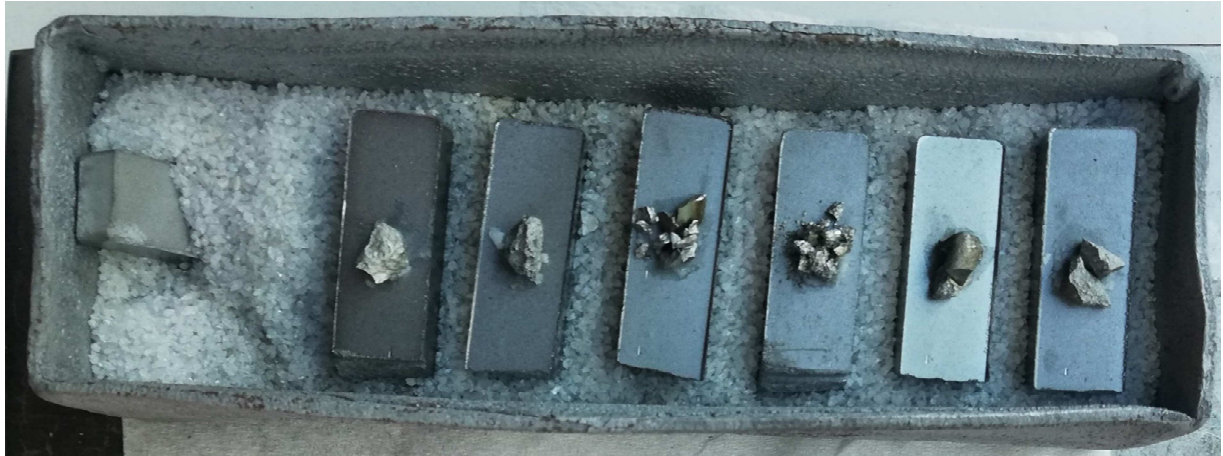
Figure 15 Infiltration samples before the furnace run
