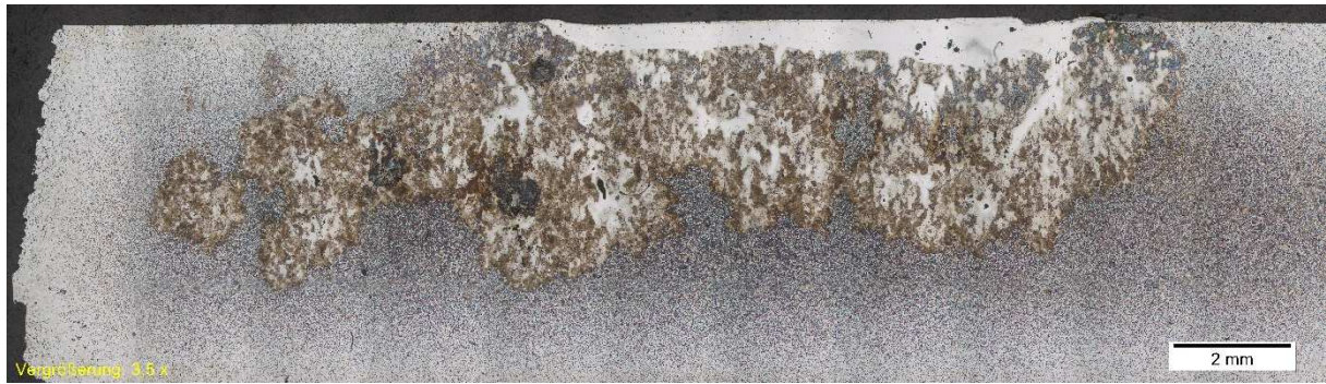
Figure 18 1% Nital etched infiltration sample under light microscope
