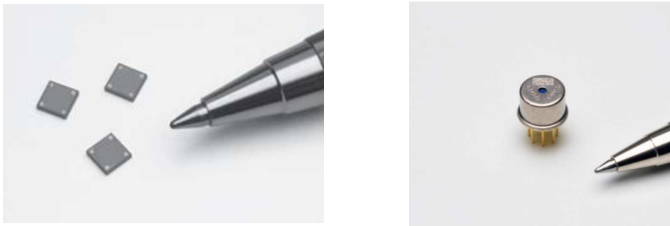
FIGURE 3.9: Left: size of the Fabry-Pérot tunable filter chips; right: size of the whole microspectrometer.
