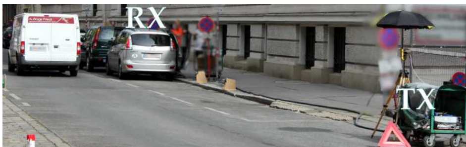
Figure 2.7: Photograph of the measurement site. The transmitter and receiver are static and urban street traffic is driving by.
