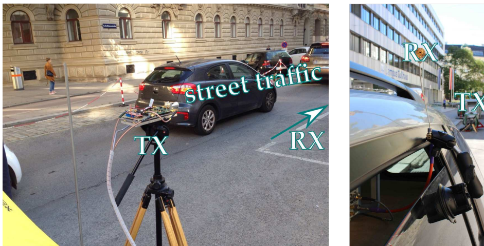
Figure 2.8: Zoomed photographs of the measurement site. On the left-hand side the photo shows the transmit horn antenna mounted on a tripod. As multiple reflection with the transmitter car are below the receiver sensitivity, the TX car is replaced with a tripod. On the right-hand side the photo shows the open-ended waveguide receive antenna mounted at roof height at the left, rear car side window.
