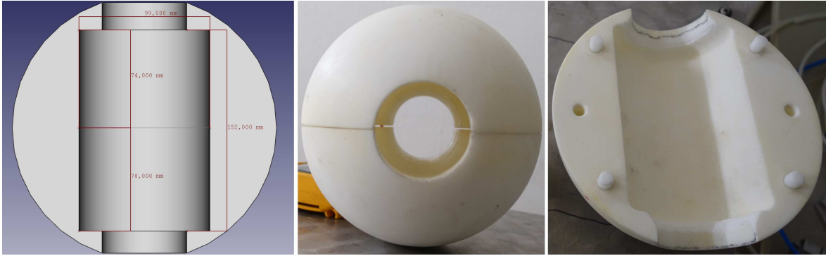
Figure 3.10: CAD drawing (left) and pictures (middle and right) of the neutron absorber used in the measurement.
