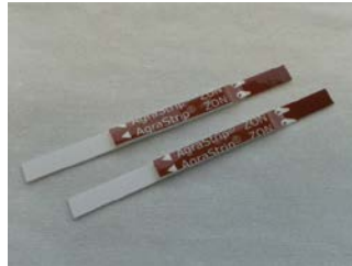
Figure 2 AgraStrip® by Romer Labs - quick test for ZEN contamination in corn samples
