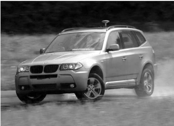
Fig. 3 SUV test vehicle performing a powerslide
