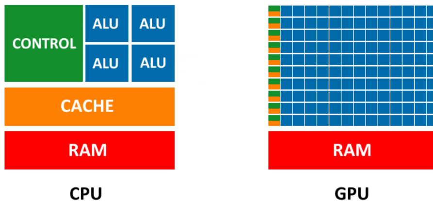
Figure 2.3: Differences between CPU and GPU
