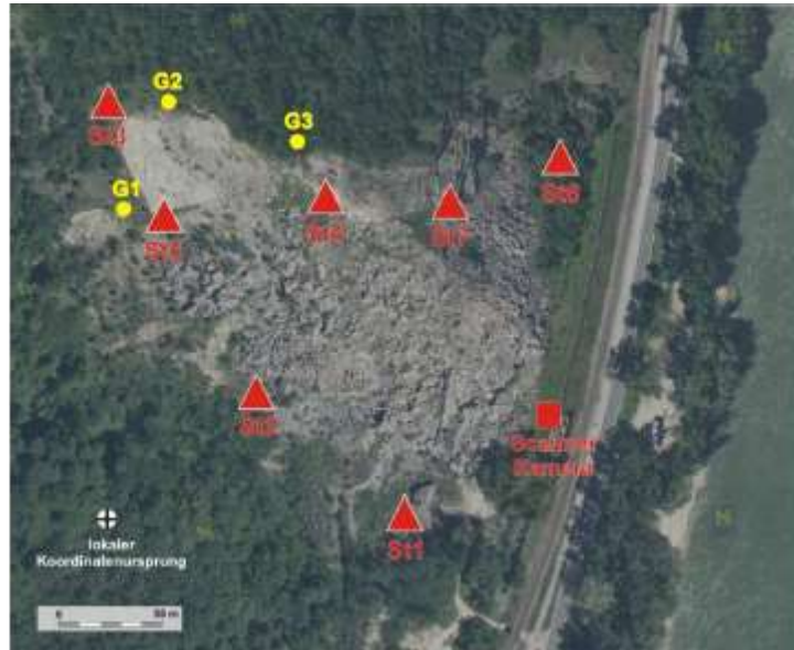
Figure 8.2. Location of seismic stations (red triangles) in a Google Map; the position of the laser scanner and the film camera are indicated by the red rectangle; a white cross marks the origin of the local system; seismic stations of existing measurement system are labelled with G1, G2 and G3 (yellow circles).
