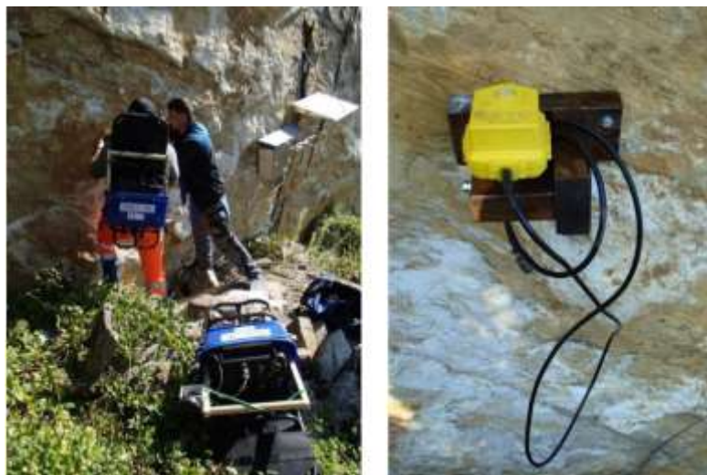
Figure 8.4. Mounting of the geophone directly on the rock of station 4.
