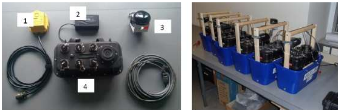
Figure 8.1. Seismic measurement system; a) Components: 1 .Geophone + cable, 2. Battery, 3. GPS antenna + Cable, 4. Recorder; b) Assembly in easy to transport and quickly installable systems.
