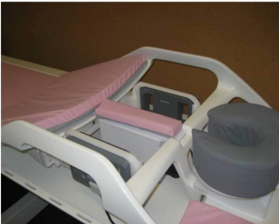
Figure 1.2: A MRI scanner and the coil used for breast imaging. Courtesy of Katja Pinker-Domenig.
