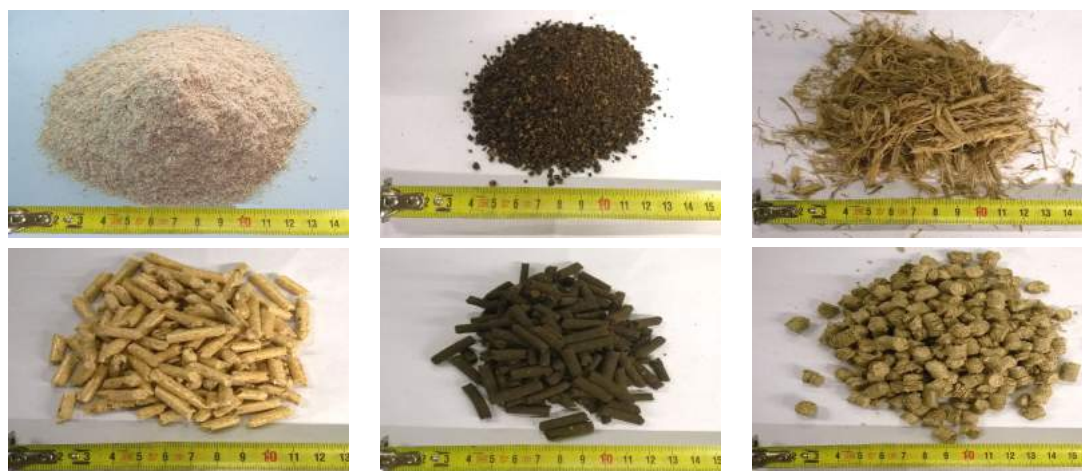
Figure 5.1: Presentation of feedstocks used in this work. Milled wood and wood pellets (left), raw EOP and pelletized EOP with \text{CaCO}_3 (middle) and chopped sugarcane bagasse and sugarcane bagasse pellets (right). In order to reach better dosing characteristics and avoid blockages in the fuel dosing system, all feedstocks were pelletized
