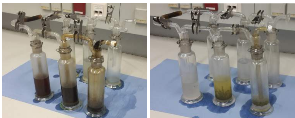
Figure 5.15: Impinger bottles after tar measurement at sampling point B (left) and sampling point A (right)
