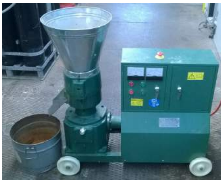
Figure 5.21: Pelletizer manufactured by company Cissonius for feedstock preparation. PP200, 7.5kW, 380V
