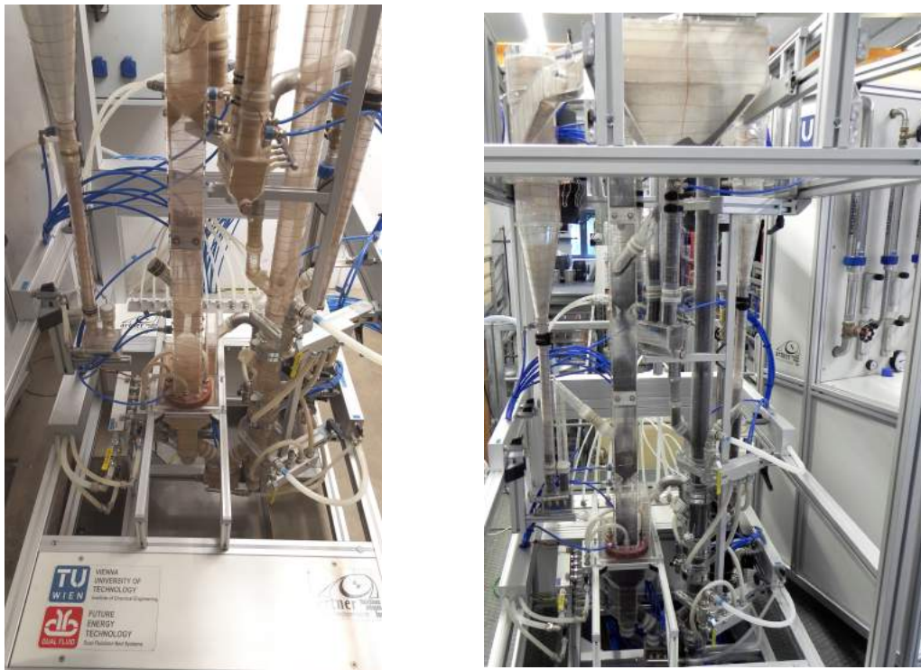
Figure 4.1: The cold flow model system is shown. Pressure indicators (blue tubes) and air inlet tubes (white tubes) are illustrated
