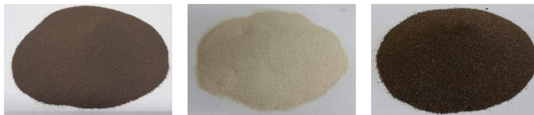
Figure 5.2: All bed materials used are shown. Fresh olivine (left), fresh limestone (middle) and a mixture of fresh olivine and fresh limestone (right)
