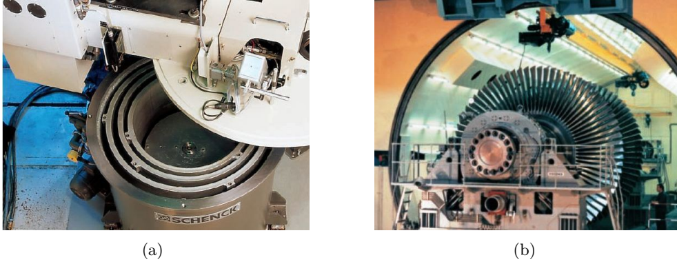
Figure 1.2: Dynamic burst test rigs with highest safety class D [50]: (a) intermediate rotor test inside four steel safety containments; (b) heavy duty rotor test inside a tunnel of 3 m thick reinforced concrete.
