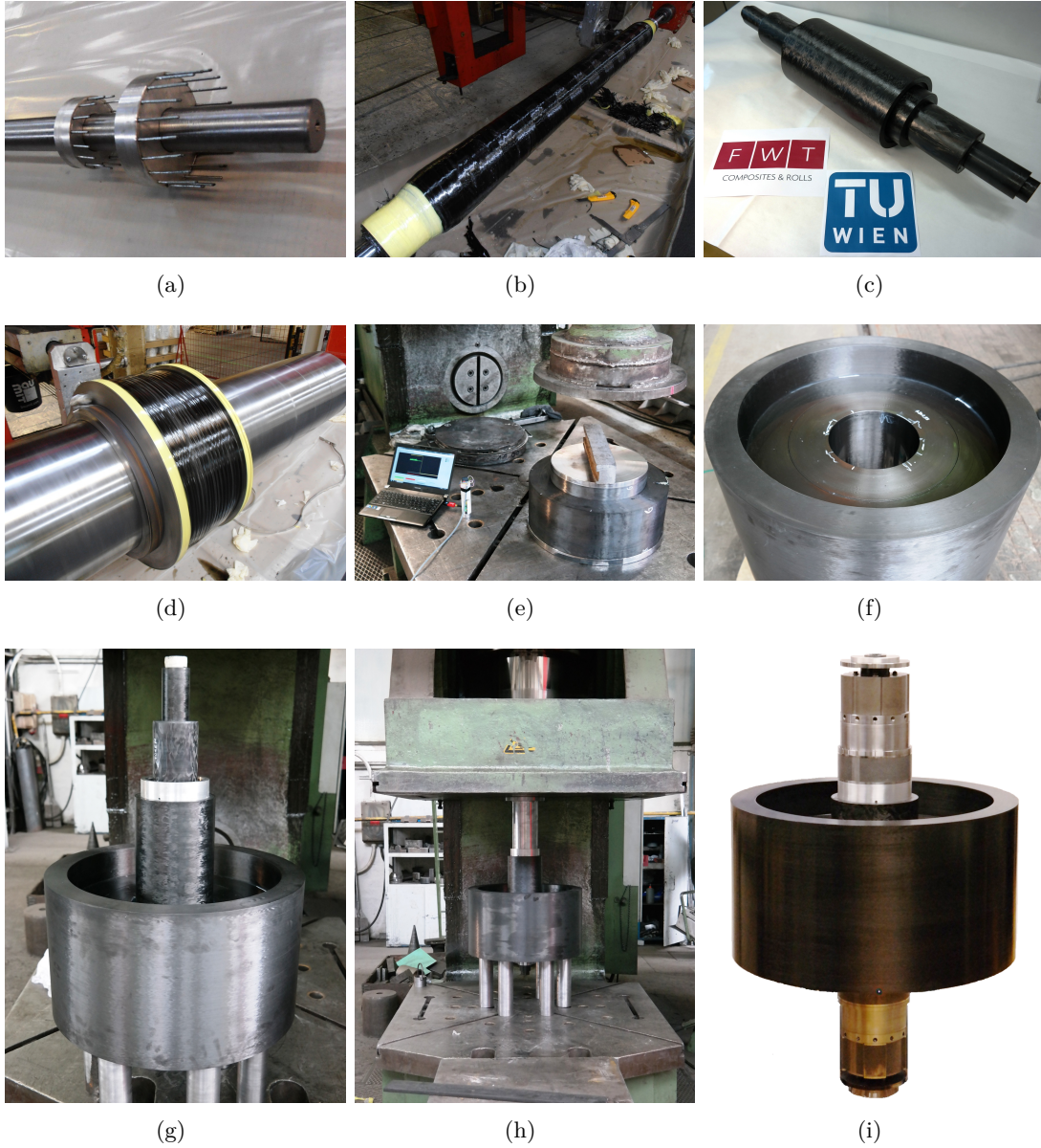
Figure 5.9: Fabrication and assembling of the FESS rotor: (a) steel mandrel with symmetric mounted winding pins; (b) winding operation of the hollow shaft; (c) finished machined shaft; (d) steel mandrel for hoop winding operation; (e) press-fitting of the rings; (f) finished machined inertia mass; (g) centric positioning of the shaft; (h) press-fitting of the shaft and the inertia mass by hydraulic press; (i) finished assembled rotor including the components of the axial and radial AMB's and the M/G.
