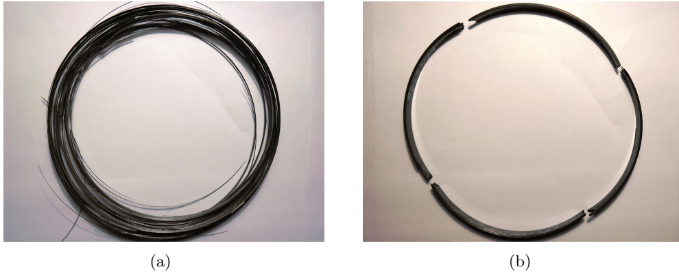
Figure 3.20: Failure of split disc test hoop wound ring specimen: (a) T800S/705; (b) K13916/705.
