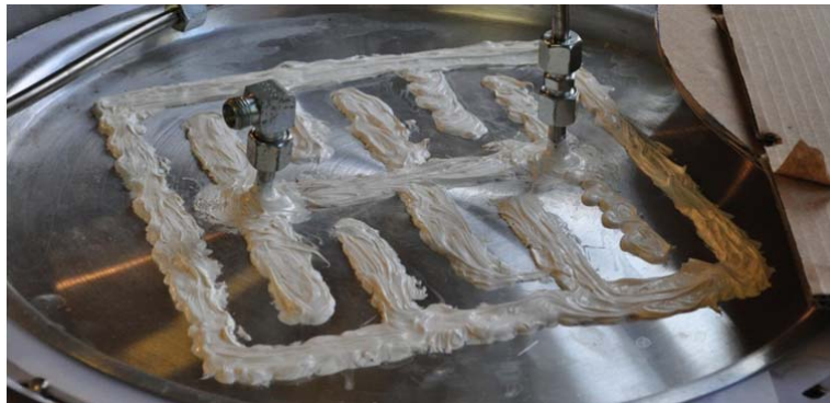
Figure 61: Evaporator seal with glue
