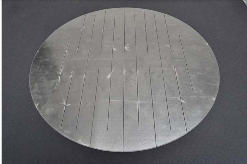
Figure 60: The aluminum evaporator sheet attachment with the special glue
