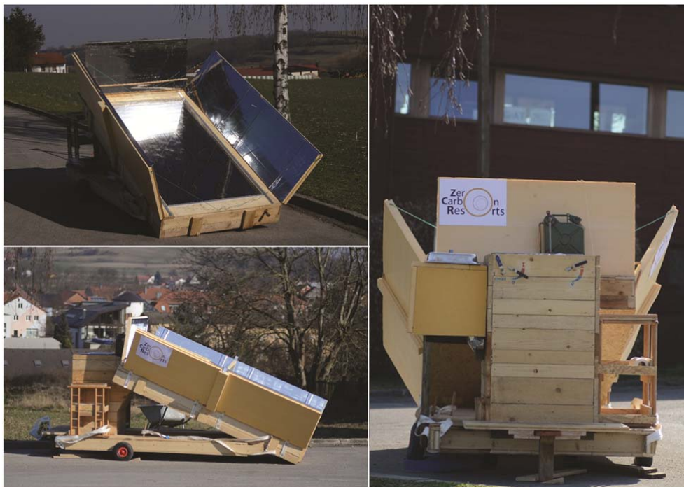
Figure 42: Prototype of solar refrigerator and solar cooking stove
