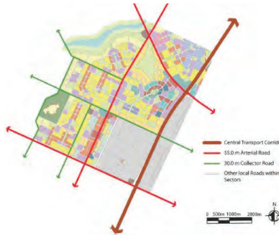
Figure 6-3: Internal Roads within Sectors and the Connectivity with the Strategic Road Network
