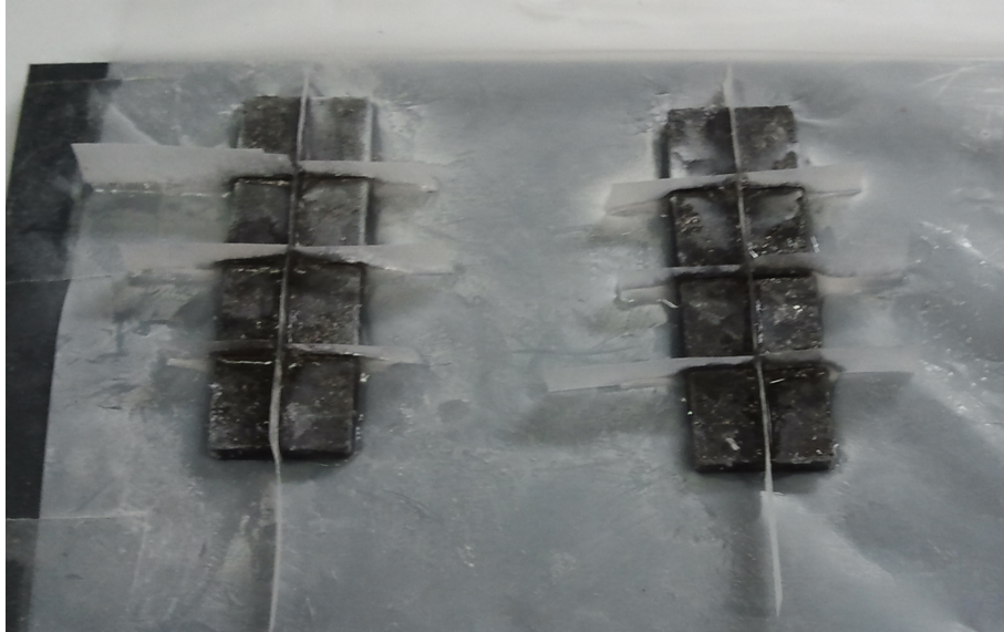
Figure 5.31: Photograph of 2 PMs composed of 8 parts during manufacturing.
