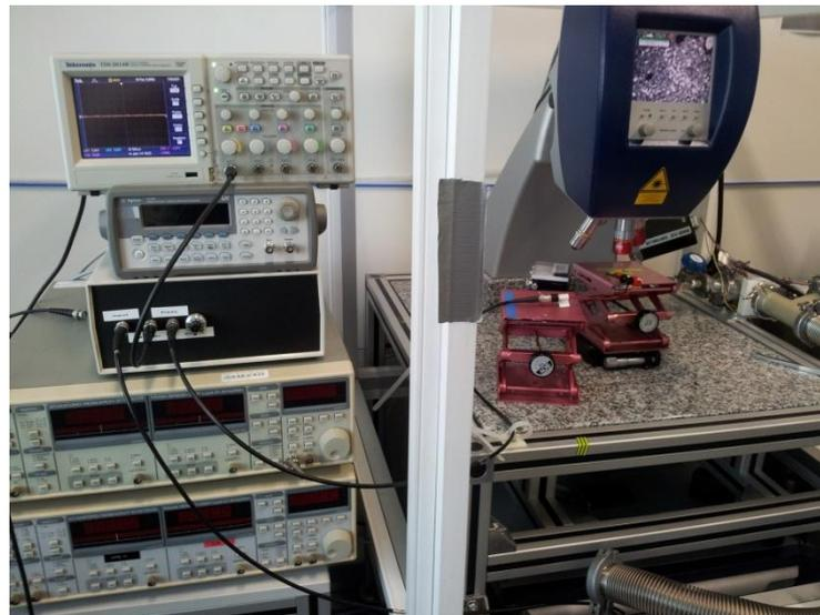
**Figure 8: Polytec Scanning Vibrometer (PSV) and oscilloscope**
