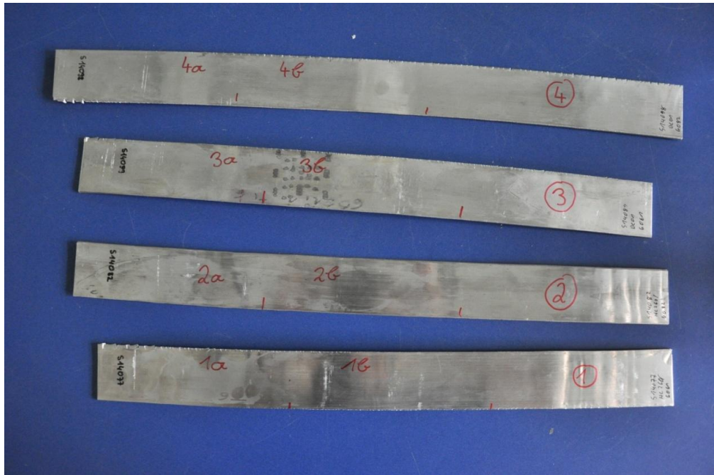
Abbildung 4-22 Probe 1 – HC260/6061; Probe 2 – HC260/6082; Probe 3 – DC01/6061; Probe 4 – DC01/6082
