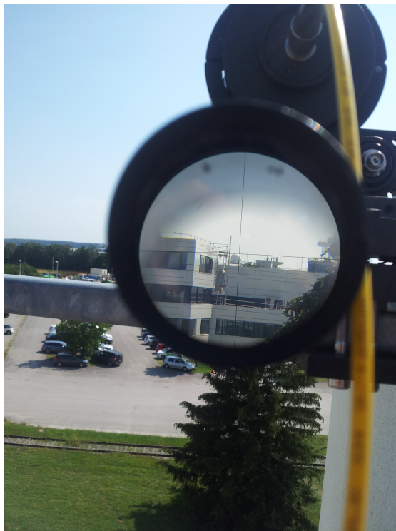
Figure 5.4: Aiming through the scope to place the beam on the primary telescope mirror.
