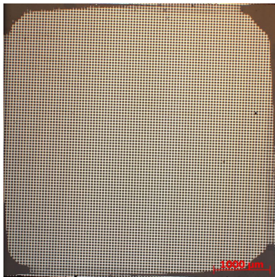
(a) Coarse current collector on LSF
