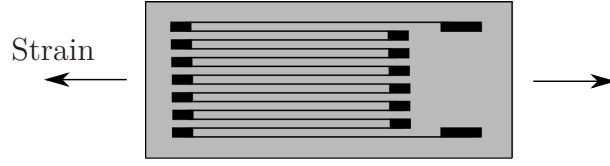
Figure 3.6: A typical arrangement of the conducting material on a thin film strain gage. High sensitivity in one direction is reached by the meanderlike structure. The figure is redrawn from [56].
