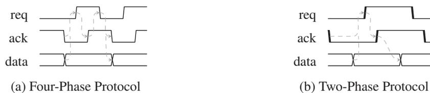
Figure 2.2: Single-Rail Protocol (Push Channel)
